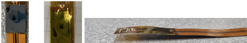
Figure 1 single diode assembled on the krypton pigtail; Pigtail for phantom studies is a 600um thick krypton strip with radiofrequency shielding. The assembling allows a certain degree of mechanical flexibility for optimal positioning of the sensor over irregular surfaces.
